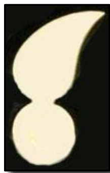
'Mouchette' is the name given to a dagger-like motif pointed at one end, and round at the other, and is typically found as a component of windows of C14 churches. Translation of the French suggests that the mason or architect who first provided its name considered it to be shaped like a little fly.
